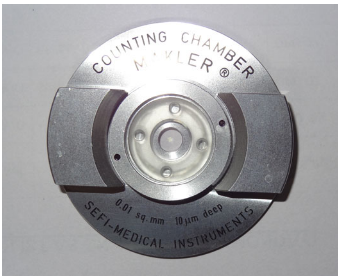
Fig. 16.1 MAKLER® counting chamber for rapid sperm analysis for counting spermatozoa. (Manufacture by SEFI Medical Instruments Ltd. Distributed by: Irvine Scientific 2511 Daimler St. Santa Ana, CA 92705)
