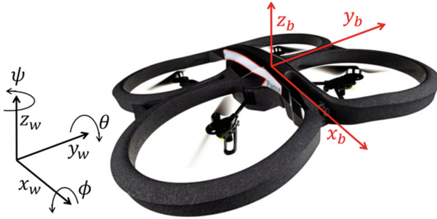
Fig. 3. Global (w) and Local (b) Coordinate systems adopted. [12]
