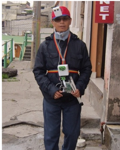
Fig. 6. A volunteer tries the prototype of the Blind Guide system.
