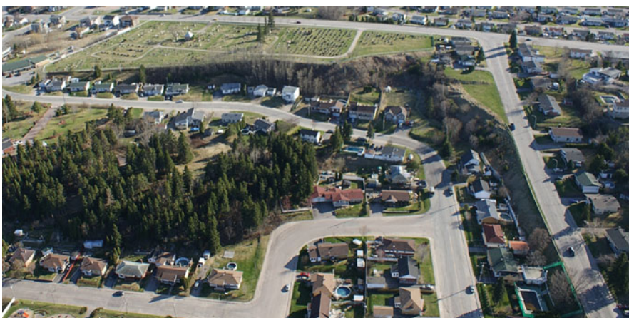
Fig. 37.1 Typical example of a slopes without erosion formed by the scarp of a large retrogressive landslide scar
