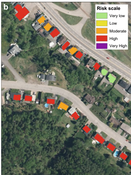
Fig. 37.4 (a) Graph of the specific risk analysis for the shallow landslide hazard; (b) Risk map example; (c) Inspection map example
