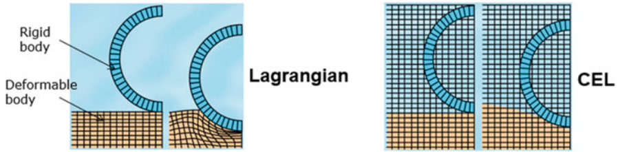
Fig. 31.1 Illustration of deformed mesh obtained from Lagrangian analysis and CEL analysis
