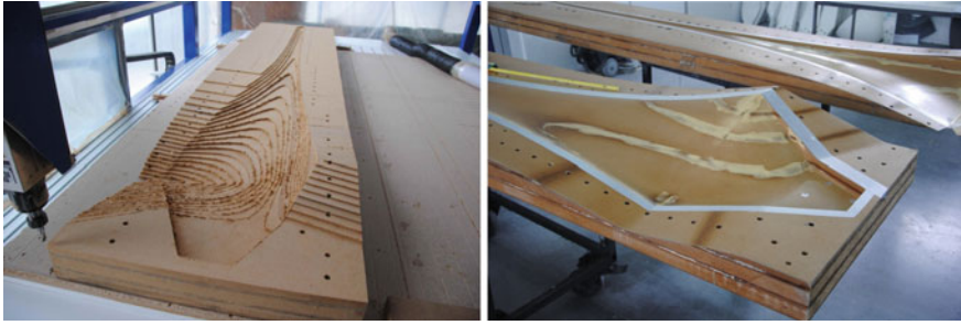
Fig. 7 Rough machining of the lower part of the mould and finished wind turbine blade mould
