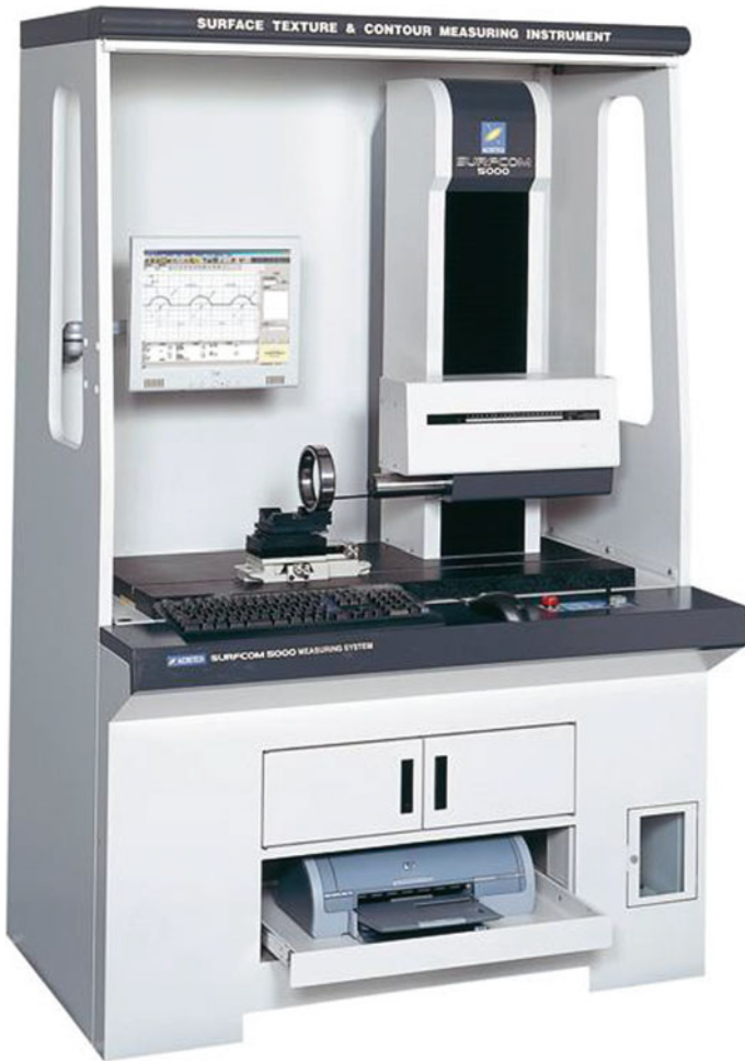
Fig. 3 Surface roughness measuring device [19]
