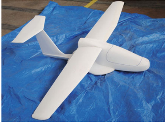
Fig. 3 Produced model of the light amphibian aircraft
