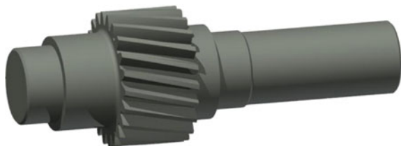
Fig. 7 3D model of pinion shaft of reduction first step
