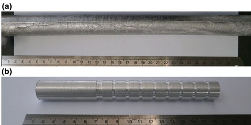
Fig. 1 a As-cast Al alloy/SSF rod; b rod prepared for cutting experiments
