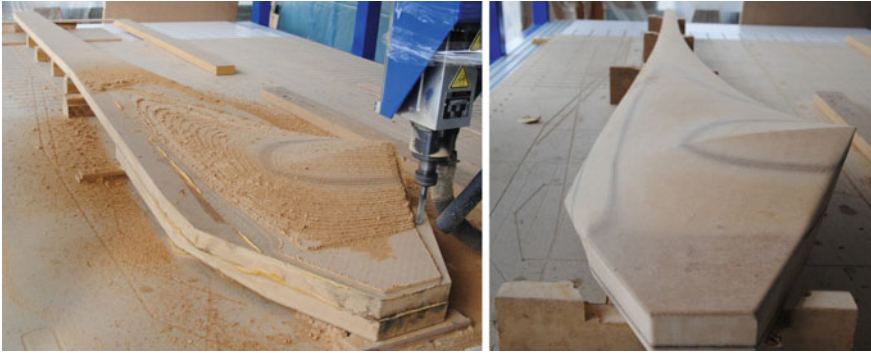
Fig. 5 Rough machining of the blade pressure side and finished wind turbine blade model
