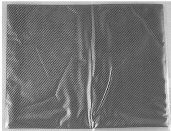
Fig. 6.17 Mud pack comprised of uranium ore dust from the Utah mine was produced by a diamond saw and enclosed in a sealed plastic envelope may deliver from 2 to 300 \mu\text{Gy/h} . Radioactivity from surface (not including alpha) is 93\% beta and 7\% gamma
