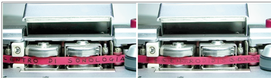
Fig. 3. Test for video shooting. On the left, a correct setting of the camera: each frame is clear and the text is readable. On the right, a wrong setting of the camera. The aim is to detect physical defects of the tape (due to aging or joints) that may correspond to a specific noise in the audio signal. Audio is directly recorded from a secondary line-out of the STUDER A-810.
