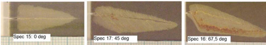
Fig. 9.33 Examples of crack path angles and delamination shapes observed for off-axis tested unidirectional GLARE2A and cross-ply GLARE3 and GLARE4B DENT specimens [44]
