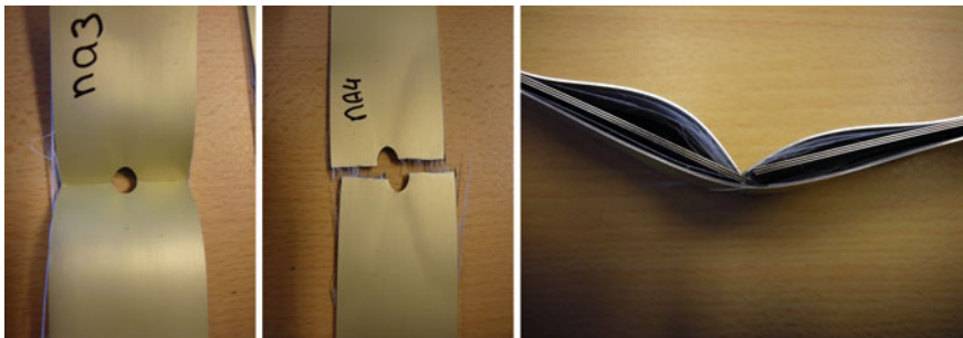
Fig. 5.9 Typical phenomena observed for the hybrid concept B1 blunt notch tests: hole ovalization, lateral aluminium layer contraction, delamination shapes as result of dynamic specimen failure and failure of inner steel-carbon plies while outer aluminium layers yield but remain intact [33]
