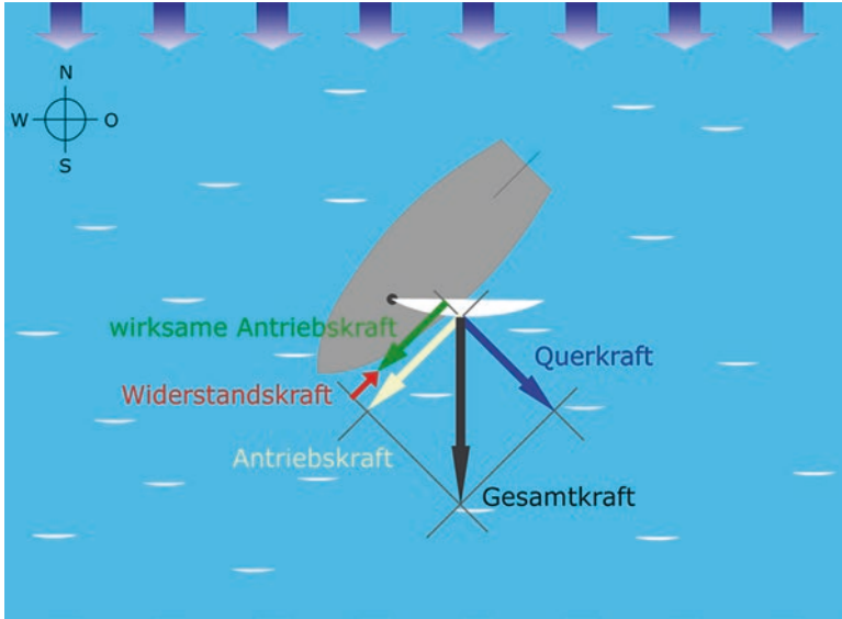
Fig. 3.1 The forces that act on a yacht in broad reach (Gesamtkraft [resultant force], Antriebskraft [driving force], Widerstandskraft [resistance force], wirksame Antriebskraft [effective driving force], Querkraft [drifting force])
