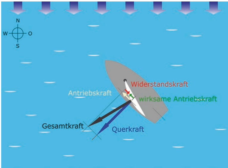
Fig. 3.2 The forces that act on a yacht in close hauled
