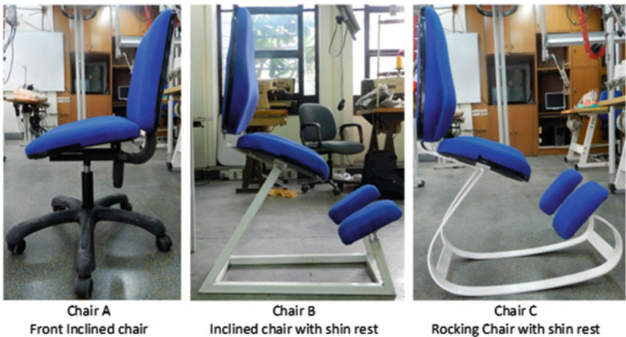
Fig. 9 Three seating workstations prototype of chair A (front inclined seat), chair B (inclined chair with shin rests) and chair C (rocking chair with shin rests)
