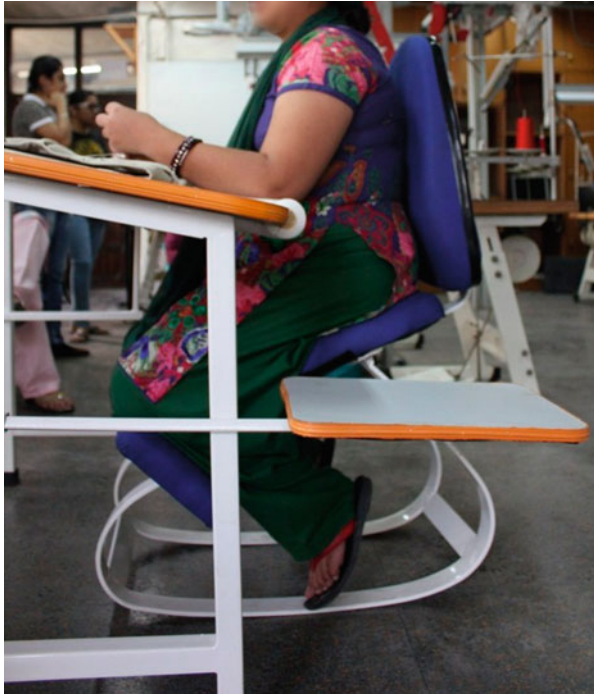
Fig. 8 Ergonomically designed sitting work station for pregnant women in finishing department of apparel industry
