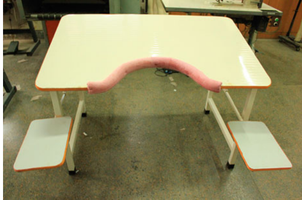
Fig. 4 Actual ergonomic table designed for pregnant women workers of finishing section
