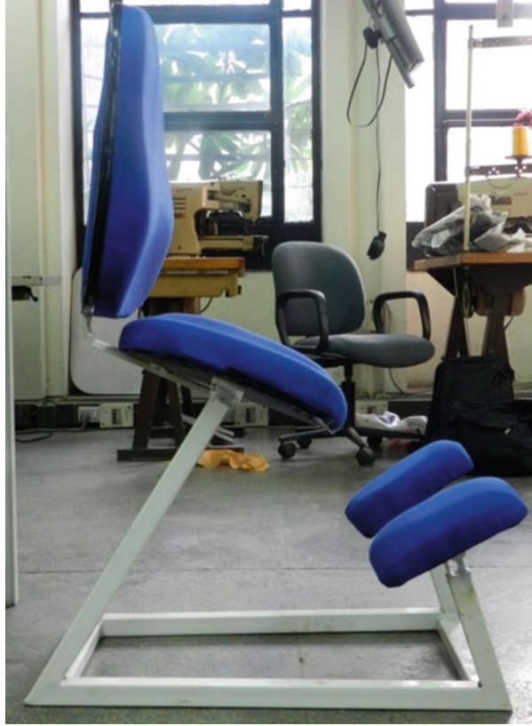
Fig. 6 Prototype of chair B with inclined seat and padded shin rests
