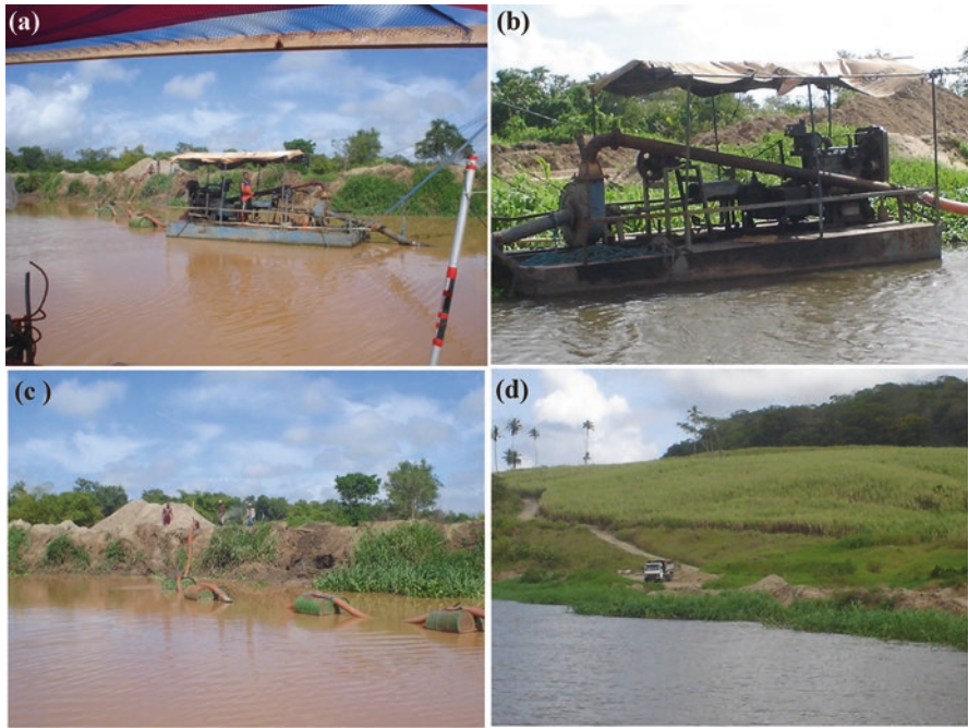
Fig. 20.12 Dredging sand in the upper portion of the Goiana River Estuary. (a) dredging; (b) dredger; (c) pumping of sand; (d) transportation to building sites
