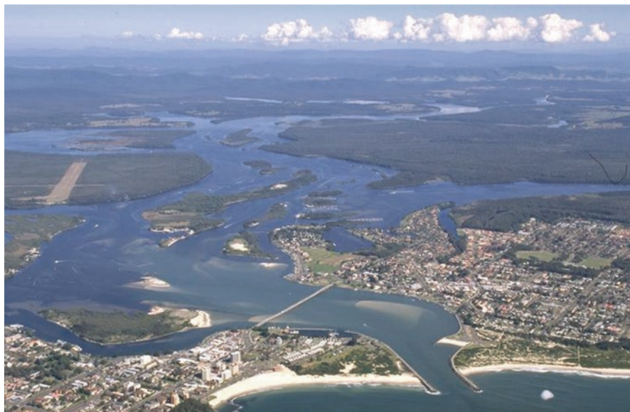
Fig. 10.11 The Wallis Lake Estuary entrance at Forster/Tuncurry, looking west (Photo courtesy NSW Government). Tidal communication between the ocean and the bay (Wallis Lake) is effected through a myriad of channels. The piling foundations for the road bridge in the foreground have been compromised severely by channel scour
