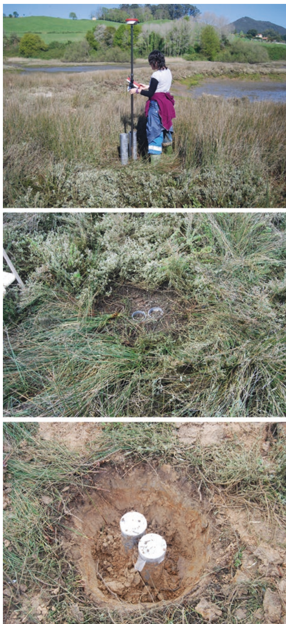
Fig. 2.2 Collection of two core replicates pushing down two PVC tubes in the Carasa salt marsh (Santofía estuary). Topographic elevation of the marsh surface is measured using a GPS-RTK
