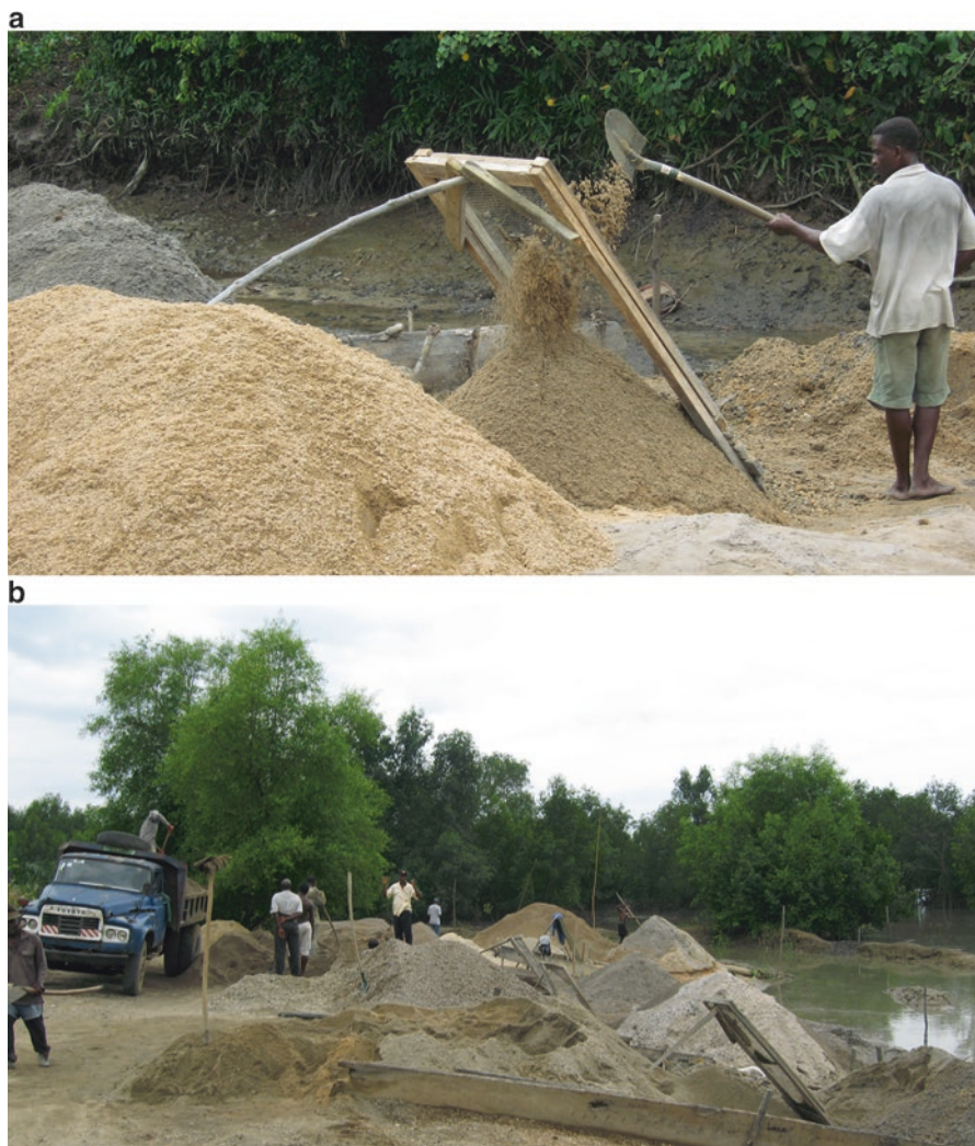
Fig. 3.10 Sand quarry in Douala degraded mangrove forest (a) partition of sands and gravels operation near a channel; (b) loading of a truck with mangrove sand near Rhizophora and Avicennia trees
