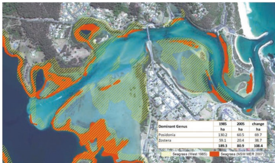
Fig. 10.32 Change in the extent of seagrass at the entrance to Lake Wagonga 1979–2005 (Duchatel et al. 2014). Loss of seagrass in the channel has been attributed to channel scour whereas on the flood tide delta it has been attributed to sand inundation
