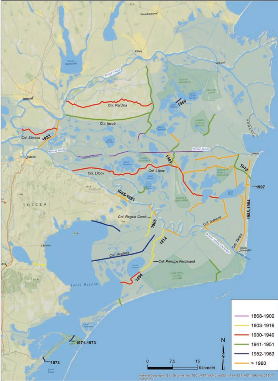
Fig. 17.2 Chronology of the hydro-technical works in the Danube Delta during the 1900–1994 period. The most important canals built during this period: Dunavat (initially called Regele Carol I) in 1907; Dranov (Ferdinand Canal) between 1912 and 1914, which connects the Sfântu Gheorghe Canal to the Razin-Sinoe Complex; Enisala (Elisabeta Canal) in 1913; Litcov (Carol II Canal) between 1929 and 1932; Crasnicol (Voievodul Mihai Canal) between 1930 and 1934; Sireasa, parallel to the Sulina Branch connecting the Sontea-Furtuna Complex to the Danube branch
