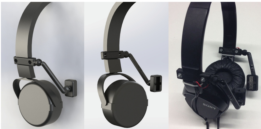
Fig. 3. Mechanical part design and integration with headphones. 3D rendering (left and centre) and real picture (right).
