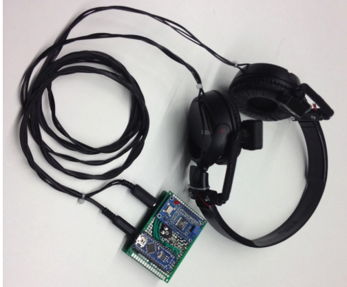
Fig. 4. Electronic device connected to the headphones and bone conductor.
