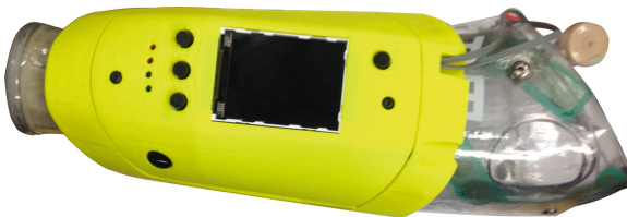
Fig. 1. Prosthesis with 3D printed housing - distal end (Left), proximal end (Right)
