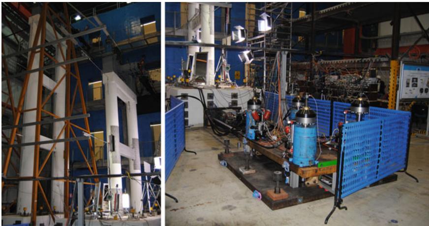
Fig. 6.4 Test set-up: global view of the piers close to the reaction walls ( left ) and FPBs test set-up ( right )
