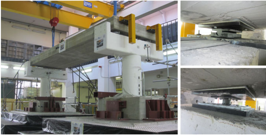
Fig. 6.10 Perspective of the test set-up ( left ), hinge and roller used as support devices ( right ) for the as-built configuration
