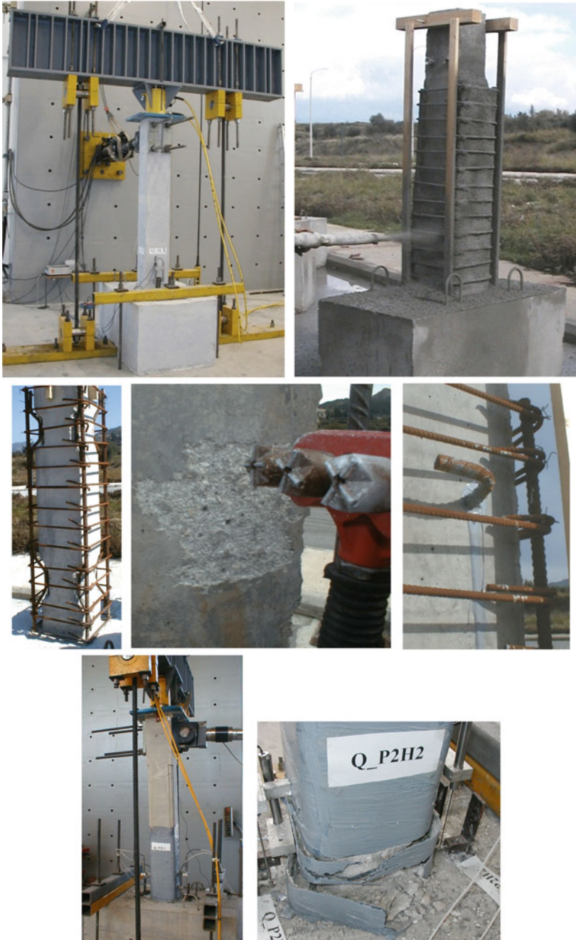
Fig. 8.1 Static testing of RC columns: original configuration ( top left ); jacketed with RC ( top right ); measures to improve interface conditions ( middle row ); jacketed with FRPs/FRP rupture ( bottom )
