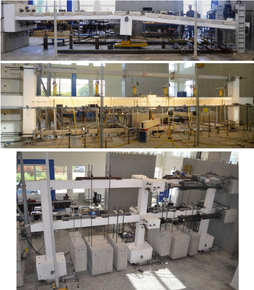
Fig. 8.4 Static testing of subassemblies for resilient systems under column-removal scenario: subassembly comprising slab portion ( top ); beam subassembly ( middle ); full scale frame tested under cyclic lateral loading ( bottom )
