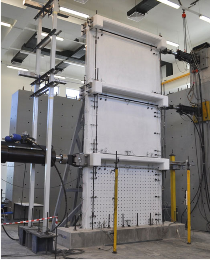
Fig. 8.2 Testing of 3-storey specimen retrofitted with TRM-jacketing
