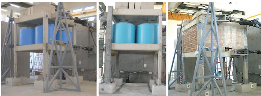
Fig. 8.6 Pseudodynamic testing of substandard structures: structure as-built ( left ), RC-jacketed structure ( middle ) and pilotis-type structure retrofitted with FRP ( right )
