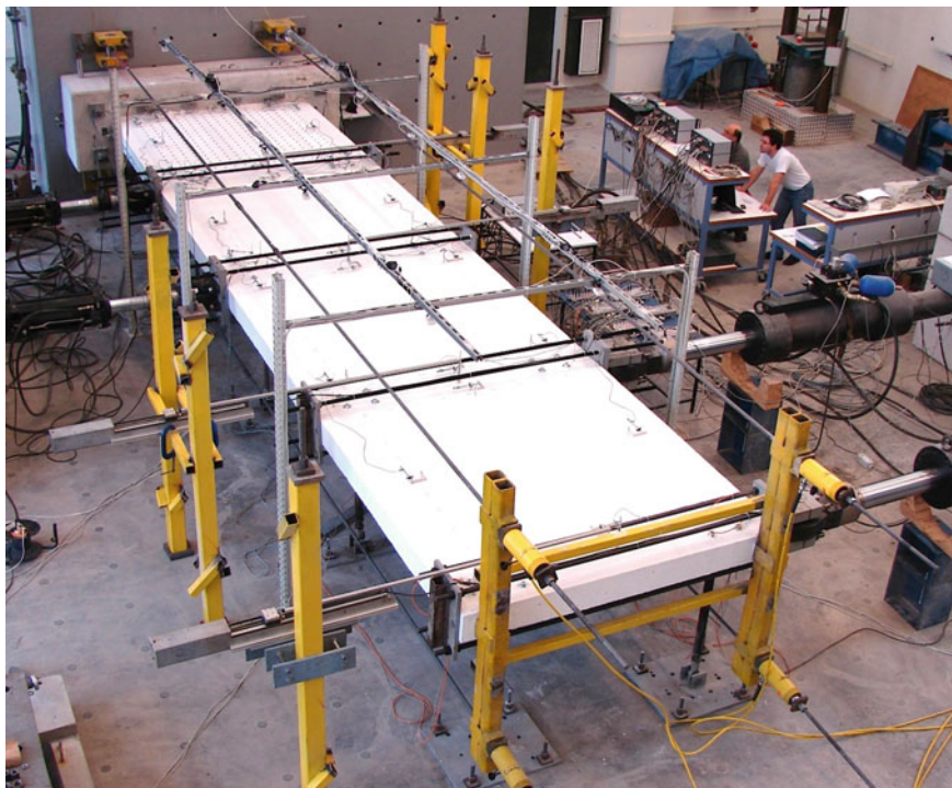
Fig. 8.7 Pseudodynamic testing of a 4-story RC infilled frame
