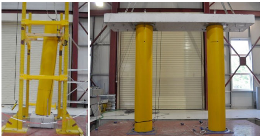
Fig. 8.5 Shake table testing of rocking structure: free-standing single pier ( left ) and freely supported rigid beam capping a pair of columns
