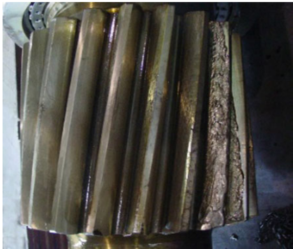
Fig. 20 The picture of the local scuffing damage
