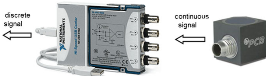
Fig. 1 The analogue-to-digital converter NI 9233 and a piezoelectric PCB accelerometer
