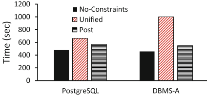
Fig. 15. Single-threaded loading in the presence of PK constraints.
