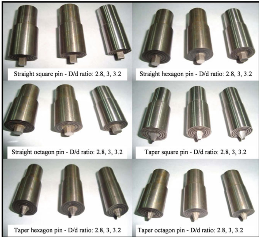
Fig. 7.13 Various FSW tools [28] with kind permission from Elsevier
