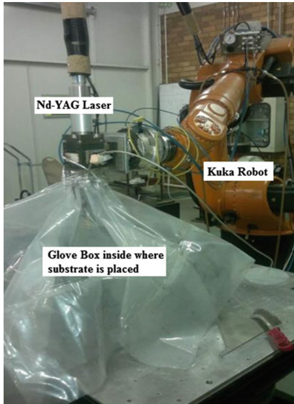
Fig. 12.7 Pictorial diagram of the LMD experimental setup
