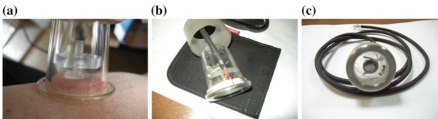
Fig. 46.10 Therapeutic head for combinational treatment of superficial tissues comprising vacuum cup (a) cylindrical piezoelement (b) and RF electrodes (c)
