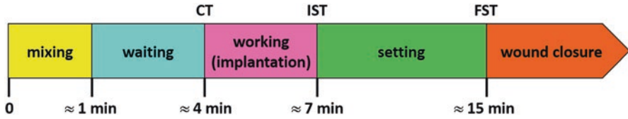
Fig. 4.5 Schematic representation of the setting process phases. CT cohesion time, IST initial setting time, FST final setting time
