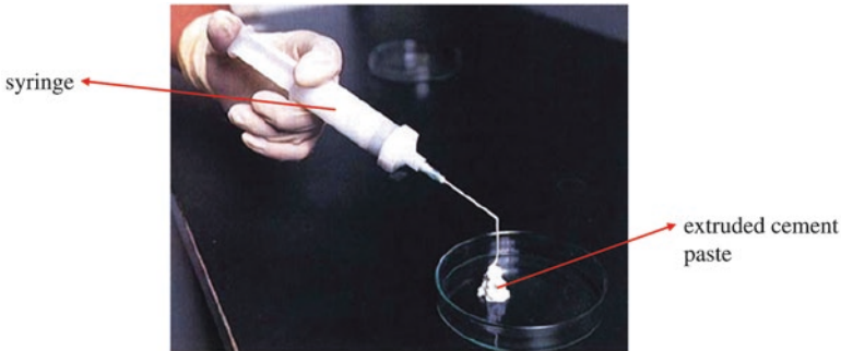
Fig. 4.11 CPCs injected using a syringe [17]
