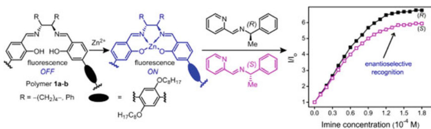
Fig. 2.6 Polymers with chiral main chain cross-linked alternately with ( R,R )-salen and 1,4-dioctyloxybenzene, as highly selective «OFF-ON» fluorescent chemosensors on Zn(II) ion, and enantioselective recognition of ( R )- and ( S )-imines under action of polymer complexes
