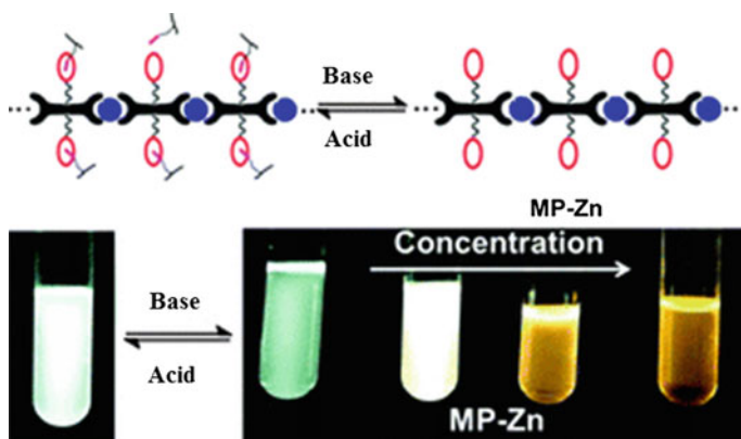
Fig. 7.9 Zn MSP, carrying dibenzo-24-crown-8 arms, which shows depending on acid-base concentration emissions [221]
