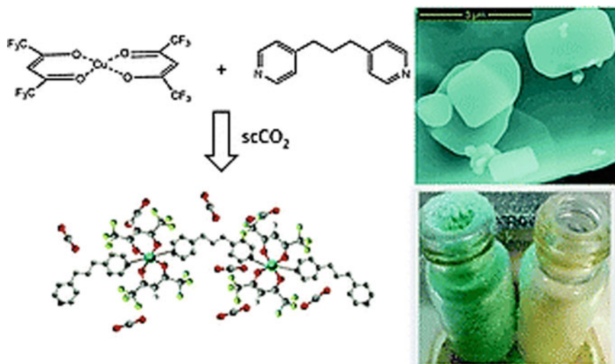
Fig. 6.52 The preparation of Cu(II) 1D MOFs using an eco-efficient method based exclusively on supercritical CO_2 as a solvent
