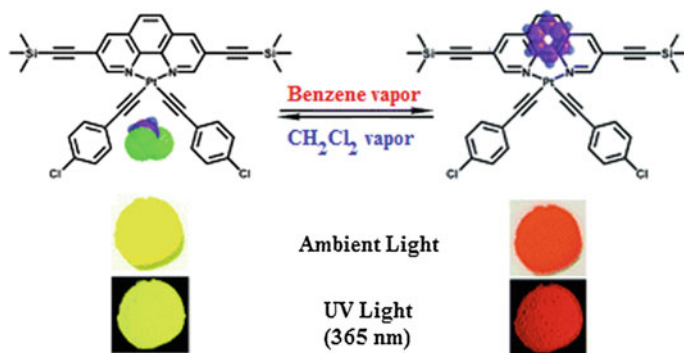
Fig. 4.34 Polymeric square-planar bis-( \sigma -acetylide) Pt(II) chelates with phen ligands as colorimetric/luminescent sensors for detecting the vapor of benzene compounds
