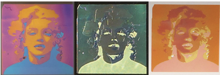
Fig. 2. Color image printed with PICSLUP ( 1 \times 1\ \text{cm} ), showing the dramatic color change according to the illumination/observation geometry. Left: Specular reflection mode ( 45^\circ:45^\circ geometry); Center: Off-specular reflection mode ( 45^\circ:0^\circ geometry); Right: Transmission mode ( 0^\circ:0^\circ geometry) [1].
