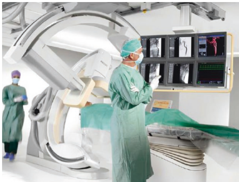
■ Fig. 11.16 Biplane neurovascular interventional lab (mock-up) featuring large field-of-view (FOV) dynamic flat-panel detectors (FDs). (See «Acknowledgments»)
