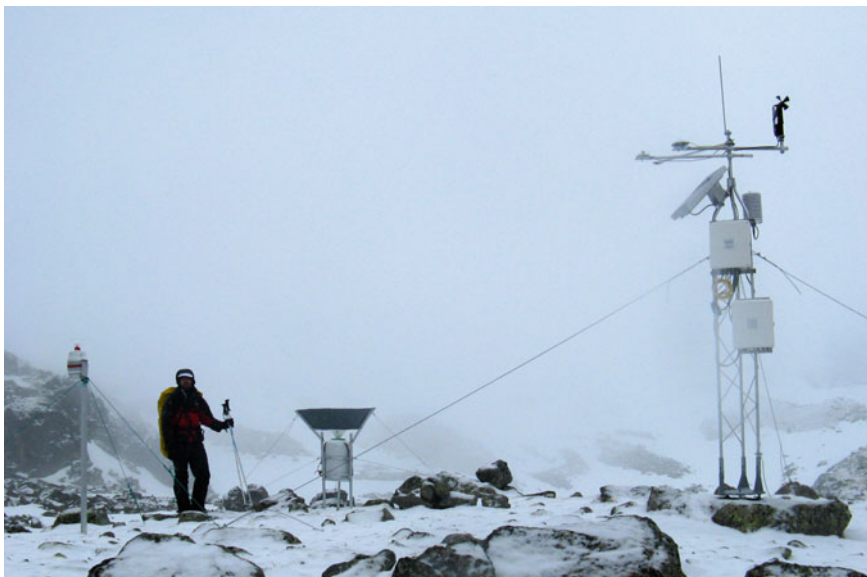
Fig. 1.1 Meteorological and atmospheric deposition monitoring station in Lake Contraix (Aigüestortes i Estany de Sant Maurici National Park (PNAESM), Pyrenees). High mountain nature reserves are particularly suitable for developing long-term studies to investigate the development and consequences of global change on ecosystems. To cope with the local characteristics of the atmospheric forcing, meteorological and deposition stations have to be deployed and maintained with a perspective of at least decades, to provide fundamental information to any other ecosystem study in the mountain catchments (Camarero 2017b). Photography: Lluís Camarero
