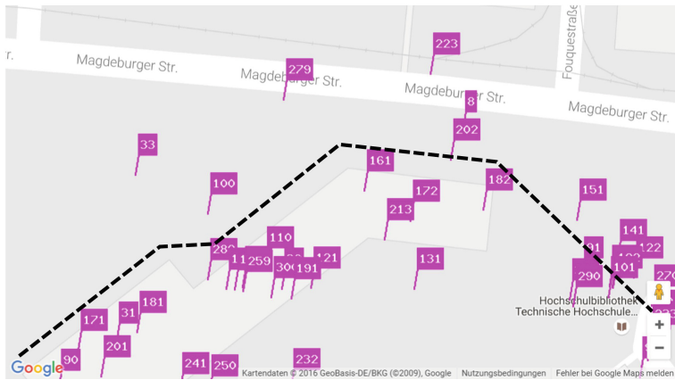
Fig. 6. The distribution of GPS positions offside the dashed line (real course) illustrate the general GPS accuracy problems.
