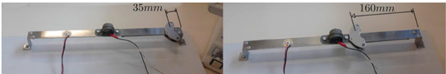
Fig. 14 Detail of placement of additional mass to emulate damage
