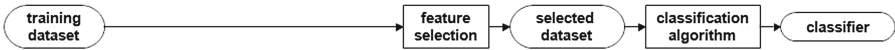
Fig. 3. The training process of classification with incomplete data by using feature selection.
