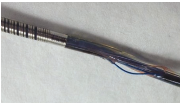
Fig. 7.4 A malfunction on a defibrillator lead. There is externalization of a high voltage conductor ( red arrow ). The insulation coating may be subject to subsequent flex failure, a high voltage short circuit between the distal and proximal conductor coil may occur. A high voltage coil is seen in close proximity to the conductor externalization. Mitigation for this externalization may take the form of taking the proximal conductor out of the circuit by programming shock vector to distal coil and can. However, the location of the external breach in conductor insulation in some cases can lead to shunting of current away from the myocardium, with the effect of leading to an increased energy requirement for successful defibrillation, even with removal of the proximal coil from the circuit
