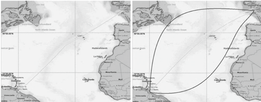
Fig. 1 Transatlantic voyage of bulk carrier from Venezuela to the English Channel within 12 days. Left side shows result from graph algorithm and right from genetic algorithm including boundaries
