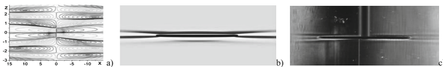
Fig. 4. The diffusion-induced flows on an obstacle with horizontal boundaries: (a) – calculated pattern of streamlines around the plate; (b, c) – patterns of density gradient field around the horizontal disc, calculated numerically and schlieren-visualized in a laboratory tank.
