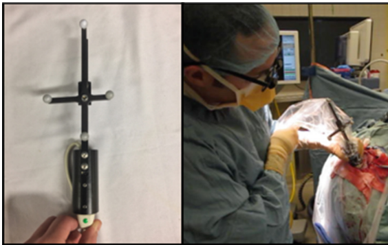
Fig. 1. Ultrasound probe with fitted tracking device (left) and use intraoperatively during neurosurgery (right).
