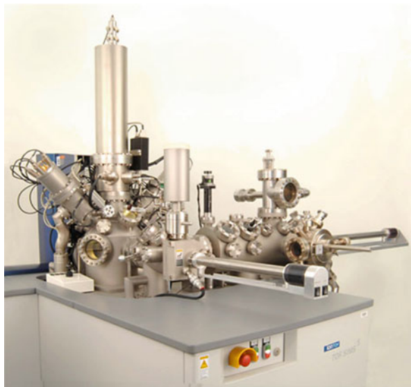
Fig. 19 A modern ToF-SIMS instrument featuring multiple ion sources and preparation chamber
