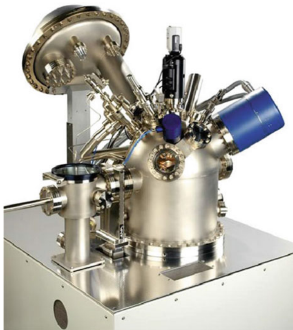
Fig. 14 Modern XPS system with serial imaging and parallel ARXPS capabilities
