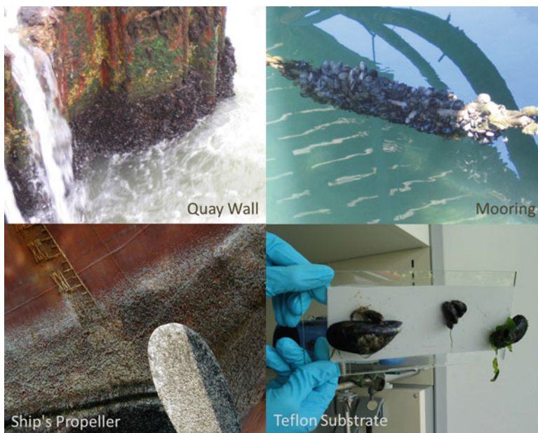
Fig. 3 Macrofouling caused by tough adherent organism, e.g., mussels and barnacles on different surfaces under harsh conditions (salinity, marine current)
