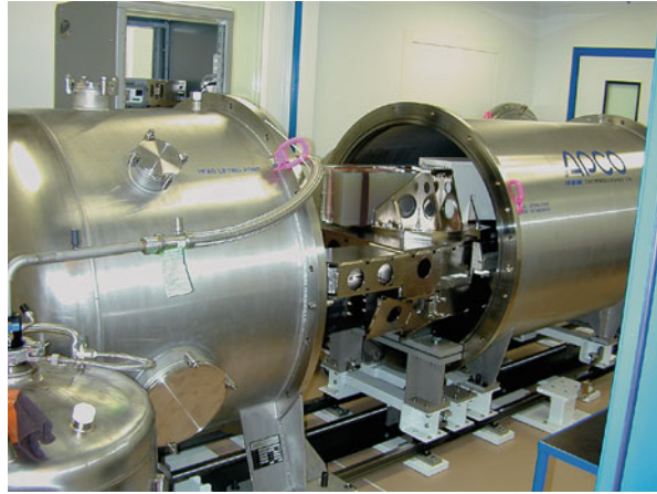
Fig. 6 View of the vacuum vessel containing the integrated spectrograph just before final closing. HARPS provided continuous operation from September 2003 to May 2015 without ever being opened
