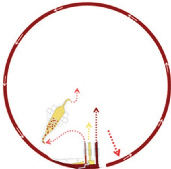
Fig. 7.3 Spectra Optia blood separation in the centrifuge using the MNC protocol. Whole blood flows counterclockwise with separation of the MNC and platelets that are drawn into the conical chamber (left) and then into the collection bag, during the harvest cycles. Platelet-poor plasma is drawn from the plasma port (center) to be returned to the patient/donor. Packed RBCs (right port) are returned to the patient/donor. (Used with permission from Terumo BCT)
