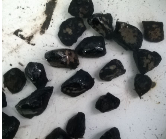
Fig. 7 Stripping of Type 1 aggregate under acidic condition pH 3 with pressure
