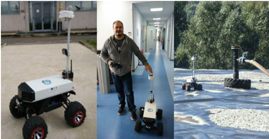
Fig. 2 Pictures of developed system during the campaign in landfill (on the right). The overall dimensions are 70 \times 50 \times 30 cm and 4 kg of weight + 2 kg of maximum payload
