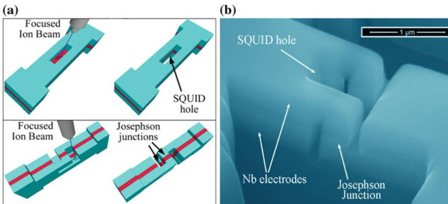
**Fig. 1** a Sketch of the main fabrication steps of a nanoSQUID. The fabrication is based on a combination of the optical lithography and Focused Ion Beam (FIB) sculpting technique. b Scanning electron micrograph of a three-dimensional nanoSQUID
