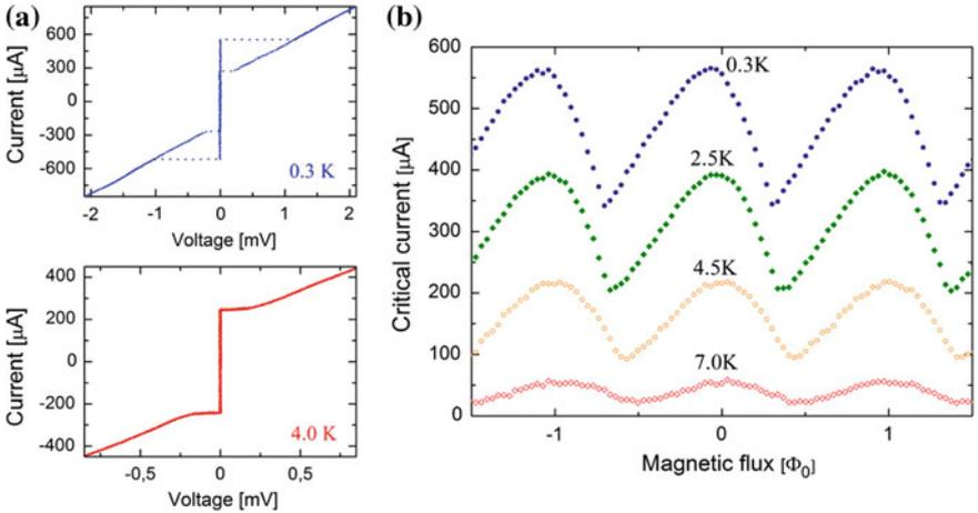
**Fig. 2** **a** Current versus voltage characteristics of a nanoSQUID measured at two different temperatures. **b** Critical current versus magnetic flux curves measured at temperature ranging from 7.0 K to 300 mK
