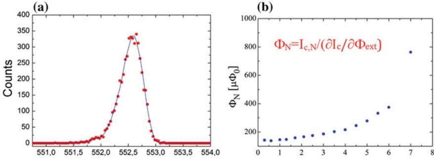
**Fig. 3** **a** Critical current switching distribution of a nanoSQUID measured at 300 mK by using the time of flight technique [11]. **b** Magnetic flux noise of the nanosensor obtained by the ratio of the critical current resolution and the current responsivity
