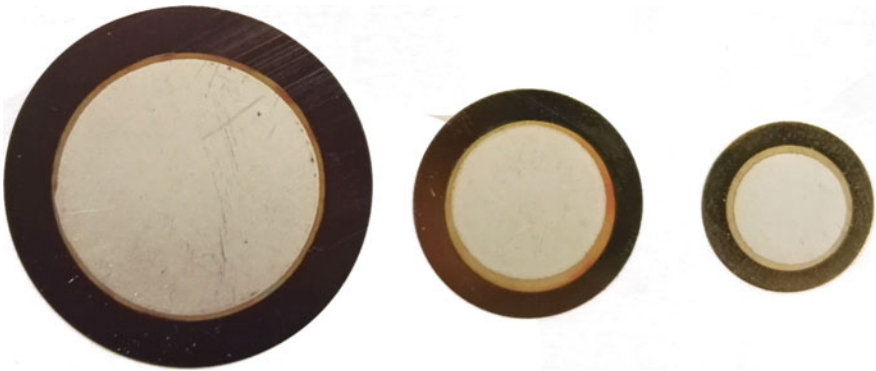
Fig. 1 Picture of the bimorphs used to develop the sensor
