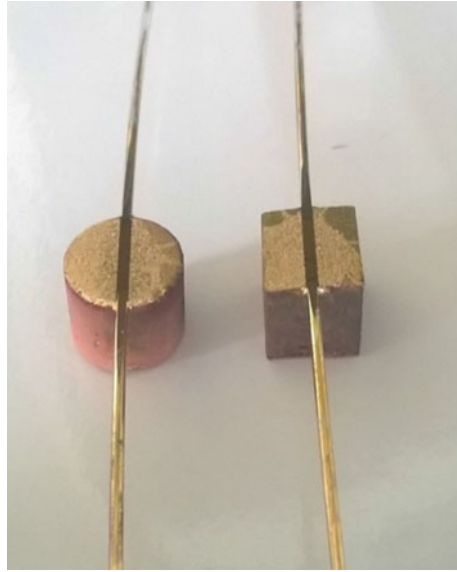
Fig. 1. Sensors with two different geometric shapes of the resin block
