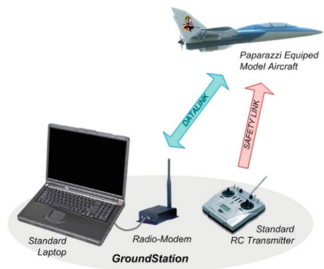
Fig. 95.2 Paparazzi UAV project overview (Available at: < https://wiki.paparazziuav.org/w/images/1/1e/Paparazzi_System_overview.jpg >. Accessed in September, 2016)
