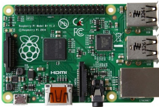
Fig. 95.1 Raspberry Pi development board Model B+ V1.2 (Available at: < https://www.raspberrypi.org/wp-content/uploads/2014/07/rsz_b-.jpg >. Accessed in September, 2016)
