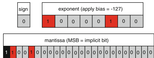
Fig. 58.1 The number 50 in single precision floating-point
