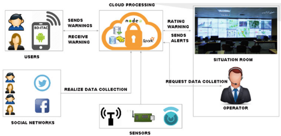
Fig. 50.11 The BD-ITAC project architecture used to run the AM
