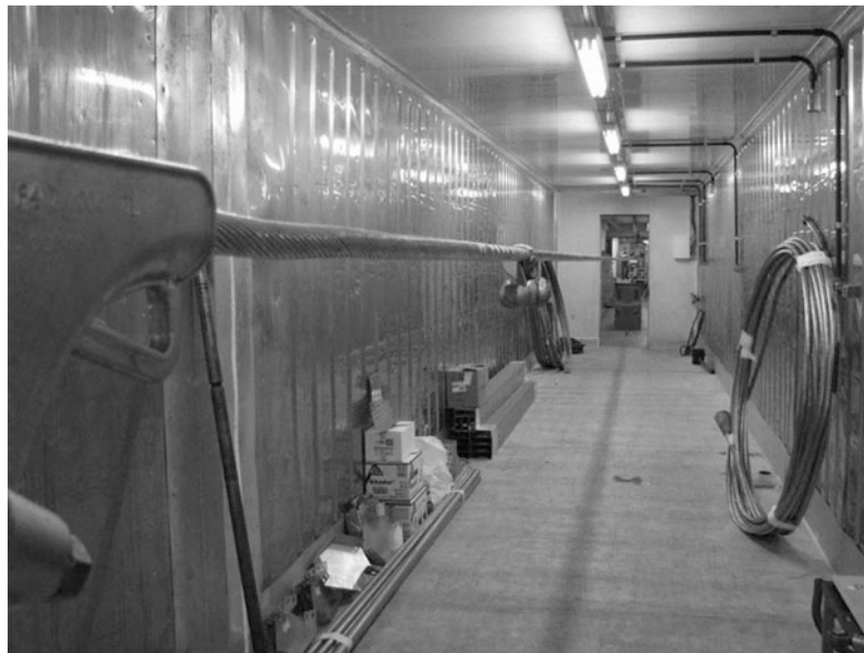
Fig. 32.1 Transmission line cable test bench
