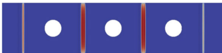
Fig. 22.6 Contact force from finite element simulation of the Hertzian beam (Courtesy of Robert Flicek)
