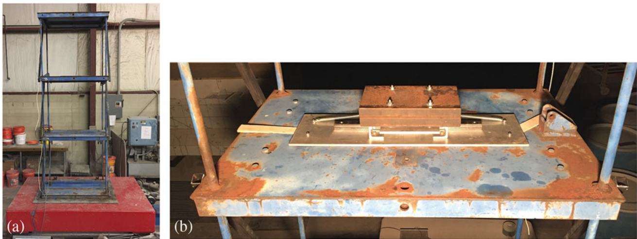
Fig. 28.1 Photos of experimental setup: (a) three-story structure and (b) floor isolation system
