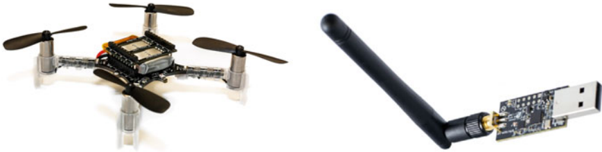
Fig. 1 Our target platform Bitcraze Crazyflie 2.0 quadcopter (left), which can be controlled from a PC using a custom USB dongle called Crazyradio PA (right). Image credit: Bitcraze AB
