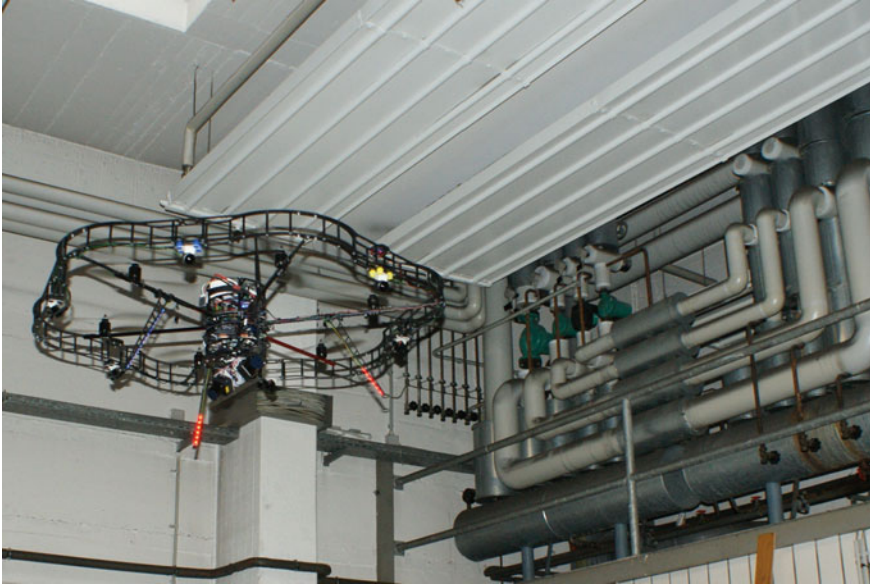
Fig. 1 Our MAV has been designed for inventory and short-range inspection tasks in indoor environments. Reliable perception of obstacles in the surrounding is key for safe operation
