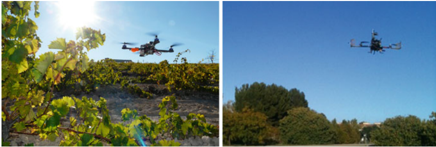
Fig. 11 The ASCTEC UAVs used for the aerial surveys: The hummingbird and the pelican models
