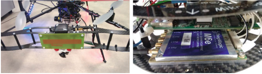
Fig. 10 RFID sensor. The MAV is equipped with a lightweight RFID antenna ( left ) and a small RFID reader module ( right ), connected to the onboard PC via USB. The RFID system is used to map positions of RFID tags in the allocentric map attached to shelves or inventory
