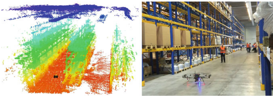
Fig. 11 SLAM point cloud. Left Resulting point cloud after pose graph optimization acquired by a manual flight along a warehouse aisle (color depicts height). Right Photo of the mapped aisle
