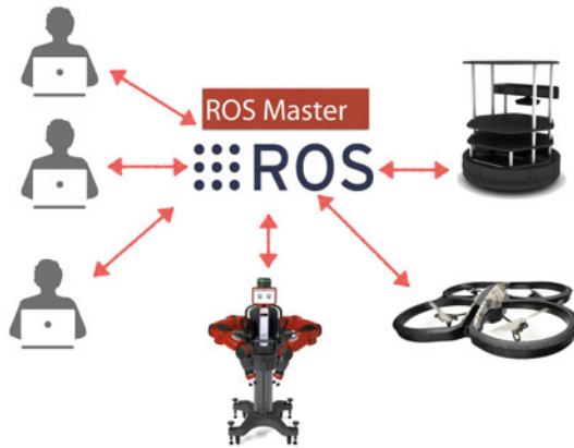
(b) Centralized Approach: One central ROS Master to which all robots and users connected. This solution is not scalable, does not provide effective management of robots and users.
