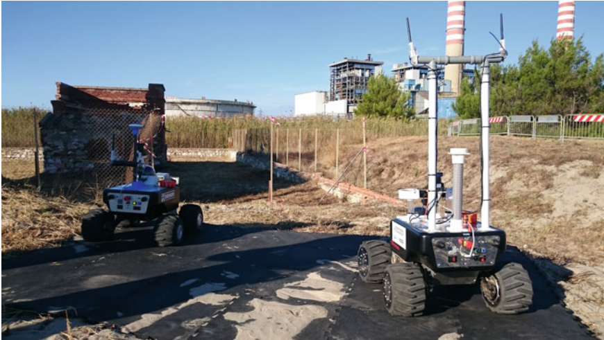
Fig. 4 The Summit XL® robotic platform with the sensors
