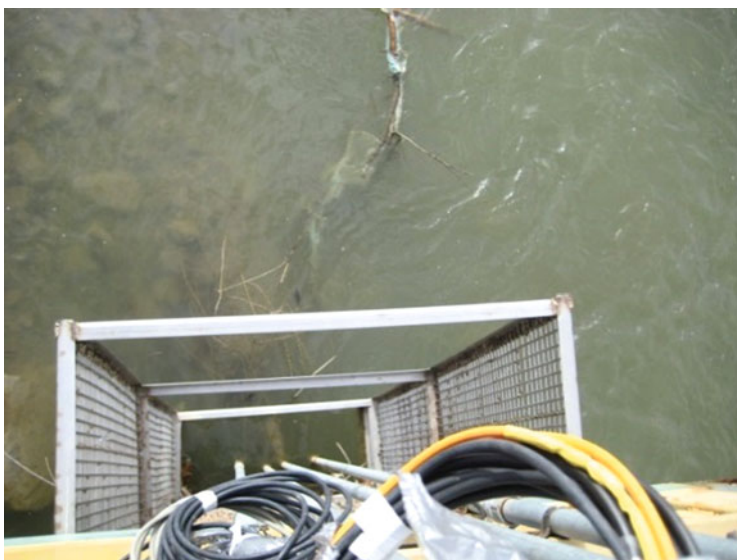
Fig. 9.4 Sensor chamber, online station Chamasean
