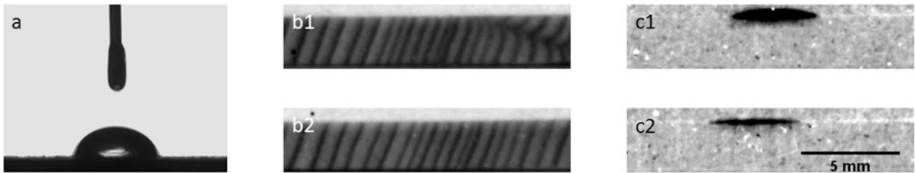
Fig. 9.2 Neutron based images showing (a) the initial varnish droplet on the wood surface, (b) the TR-wood-cross-section before the application of a varnish droplet on a blank (b1) and a pretreated surface (b2), the difference in moisture content five minutes after the application of a varnish droplet on a blank (c1) and a pretreated surface (c2)
