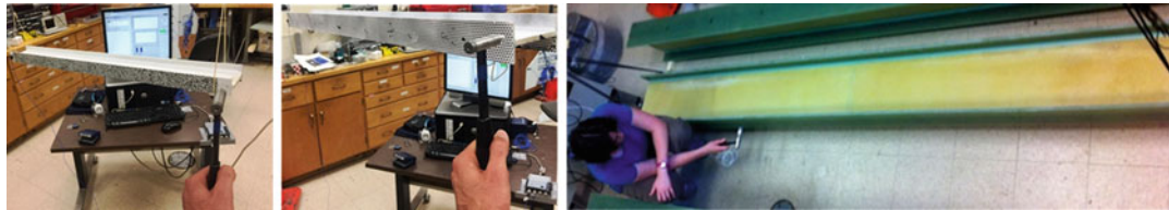
Fig. 21.3 Hammer impact test on the small ( left ), medium ( middle ) and large ( right ) beams
