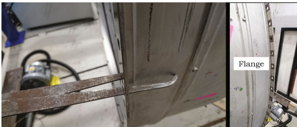
Fig. 34.3 Measurement of the casing thickness
