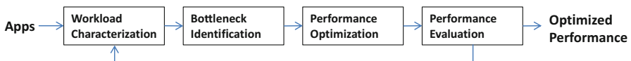
Fig. 1.3 Iterative process for performance scaling: (1) workload characterization, (2) bottleneck identification, (3) performance optimization, and (4) performance evaluation
