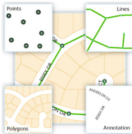
Fig. 10.11 Models of objects in vector format (source ESRI 2013)
