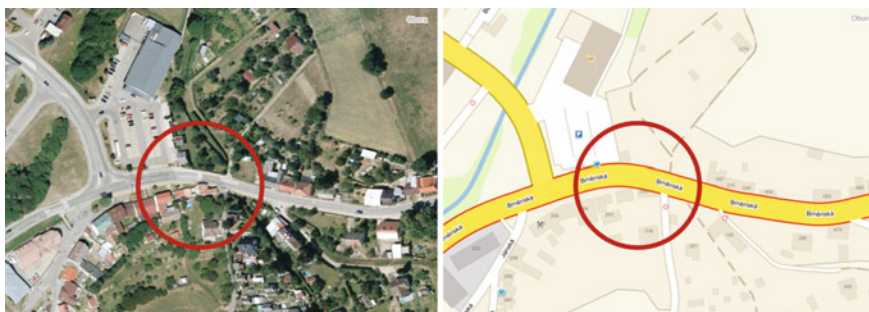
Fig. 10.30 Example of not solving conflicts between buildings and a road—see detail in the circle ( https://mapy.cz/zakladni?x=16.0779898&y=49.5613568&z=18 as of 12/8/2016)
