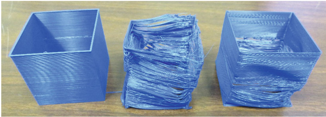
Fig. 14.4 (left to right) Healthy, faulted, and pseudo-static control corrected parts
