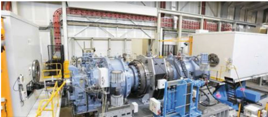
Fig. 9.14 Measurement setup for the wind turbine gearbox in the test rig configuration
