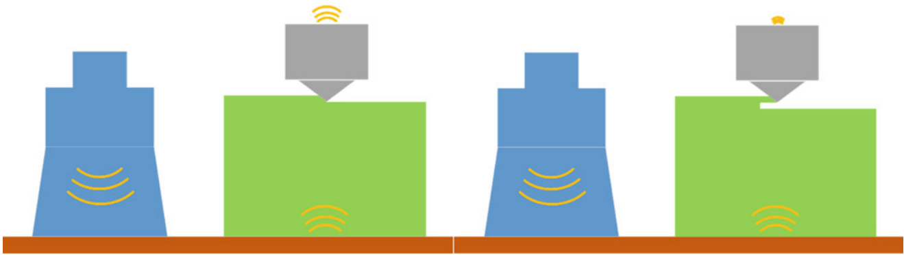
Fig. 14.5 Schematic concept for healthy ( left ) vs faulted ( right ) signal energy transmission
