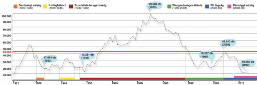
Fig. 1 Construction of new buildings in Hungary (orange—great depression, yellow—World War II, brown—socialist planned economy, green—introduction of market economy, blue—EU membership, pink—financial crisis) (Color figure online)
