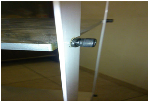
Fig. 31.5 Loose screw detail and impulse response of damaged structure
