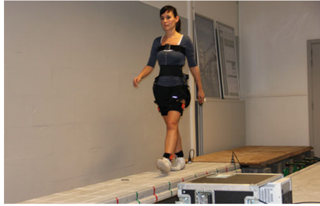
Fig. 44.1 The hollow-core pre-stressed concrete slab excited by a single pedestrian
