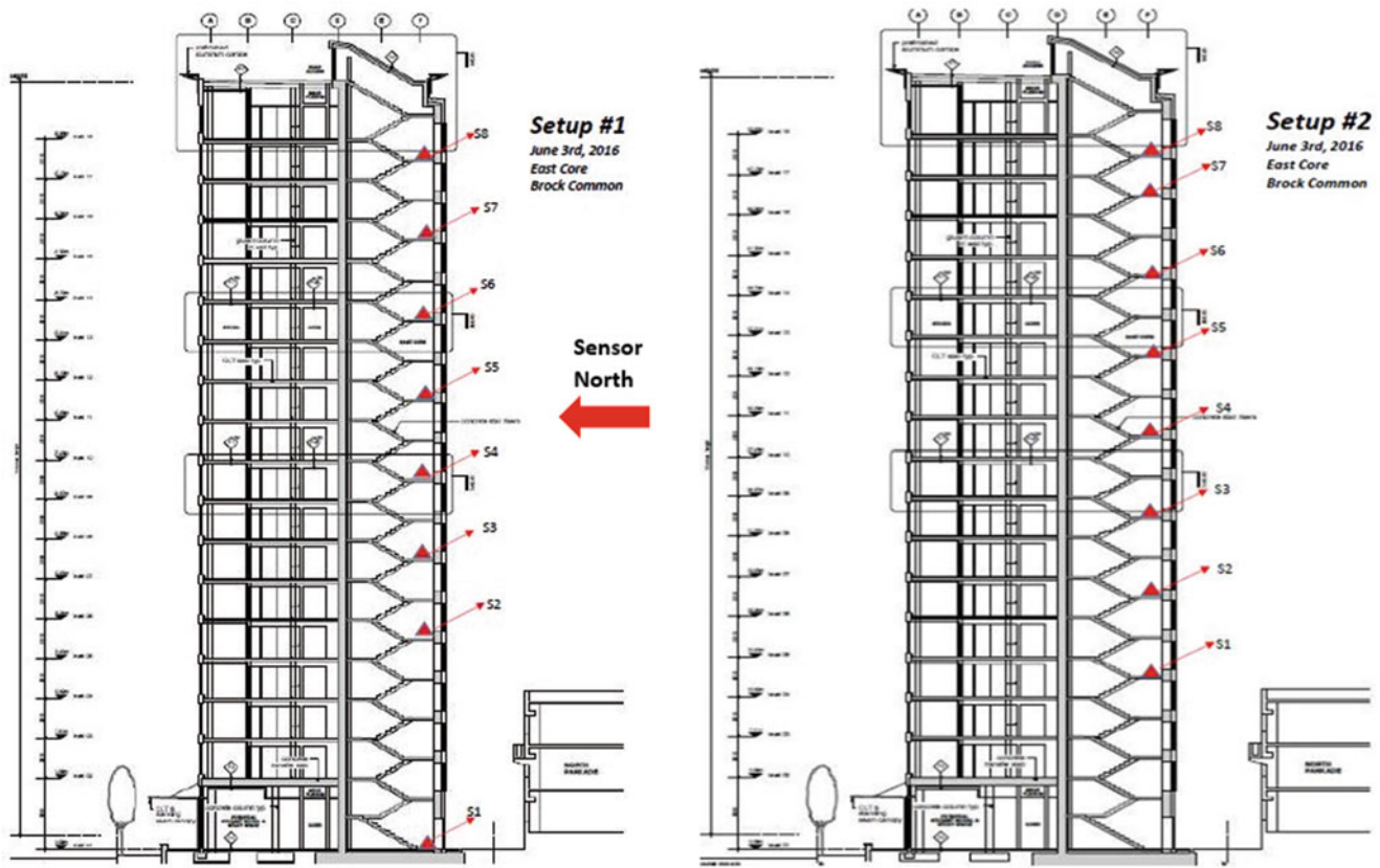
Fig. 39.2 Sensor locations and orientations along the height of the building for Setup 1 & 2
