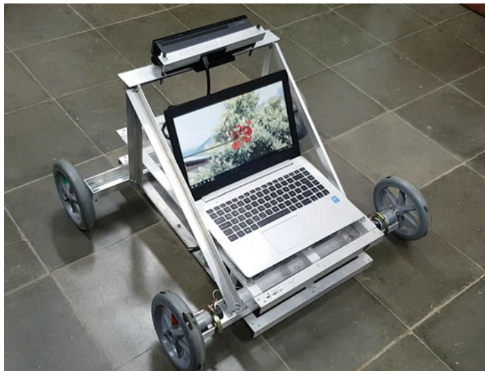
Fig. 20.1 Picture of the mobile platform carrying the computer and the MS Kinect sensor (at the top)
