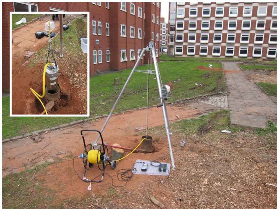
Fig. 7.4 Borehole vibration survey
