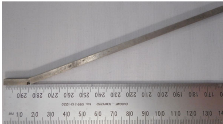
Fig. 34.4 Test coupon post-testing showing angle of deflection used as metric for damage
