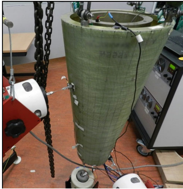
Fig. 1.1 The Modal Analysis Test Vehicle (MATV) subjected to a modal test
