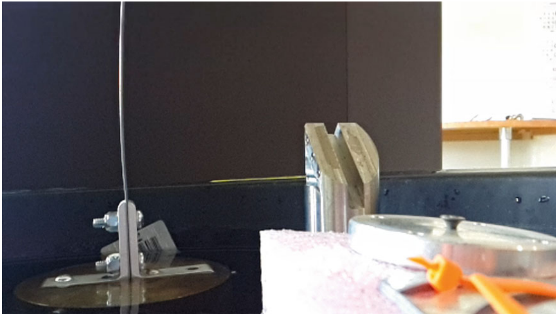
Fig. 10.1 The experimental setup of the cantilever beam floating on the water
