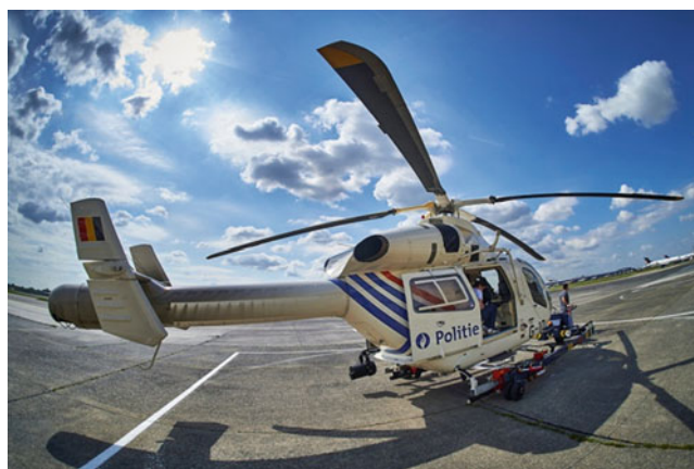
Fig. 21.2 MD 902 Helicopter with NOTAR (“NO Tail Rotor”) system
